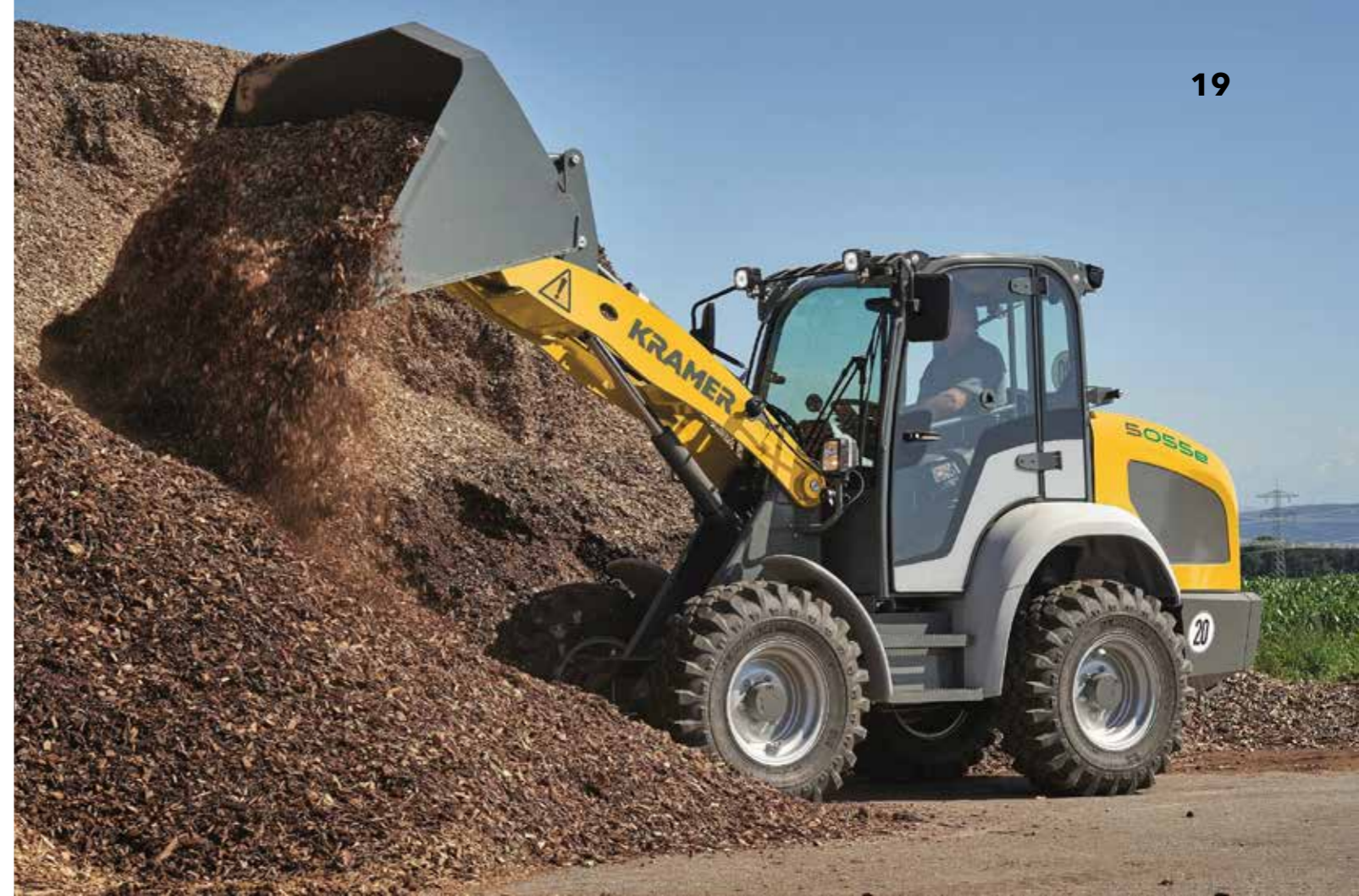
The Kramer 5055e is a fully electric, four-wheel steer wheel loader. The battery charge is enough for a day shift
